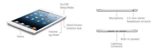
**PREPARE THE IPAD MINI** Power the unit ON using the small button on the top right side (see image above.) If the screen goes dark, press the HOME button on the bottom once to turn it back on, then swipe the arrow at the bottom to the right.
