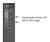
The audio monitor indicates the overall volume levels. Good audio levels will peak between -12 and -6 on the meter and will be indicated by green bars
