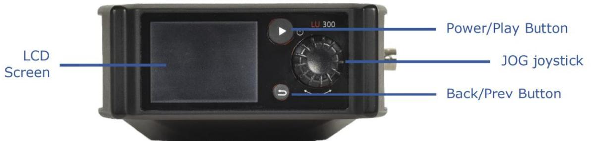
3. Turn the **LIVEU** unit on: press and hold the Power/Play button for about two seconds.
